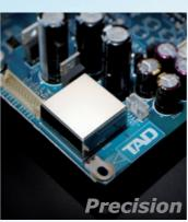
To convey all the emotion and passion of the original source, reproduction must be precise and pure. In the tradition of TAD's relentless pursuit of this philosophy, high-performance, parallel-connected, dual differential D/A converter ICs are employed—one for each channel. In addition, the Ultra-High C/N (carrier-to-noise ratio) Master Clock UPCG (ultra-high-precision crystal generator) brings the signal-to-noise
